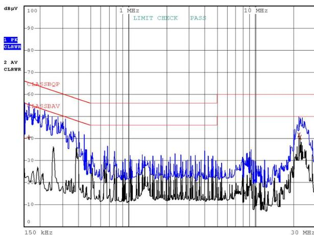
Typical phase conducted emission at 230 V<sub>AC</sub>, 50 Hz
